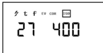
Once the film speed has been set, it is transferred to the memory of the Strobe Master and maintained when the meter is set to any operation function. It remains visible on the top right-hand side in the digital display.
